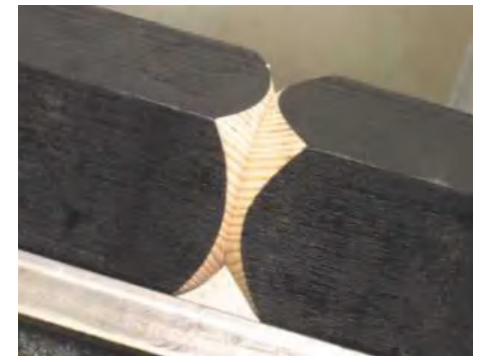
▲ Pic.12 A perfect pommel – the curve will need very little sanding as the finish off the skew is so good. The stock to the right is removed down to the round with the spindle roughing gouge
